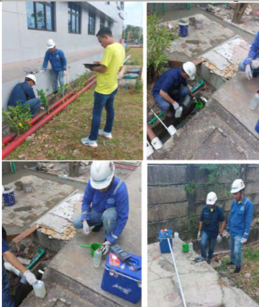
Figure 2. Waste Water Sampling at Polibatam
